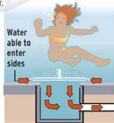
Anti-entrapment drain prevents seal
